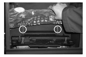
7) Place the 2 front logs on the front log locating pins. Ensure the back of both logs rest against the tabs.
